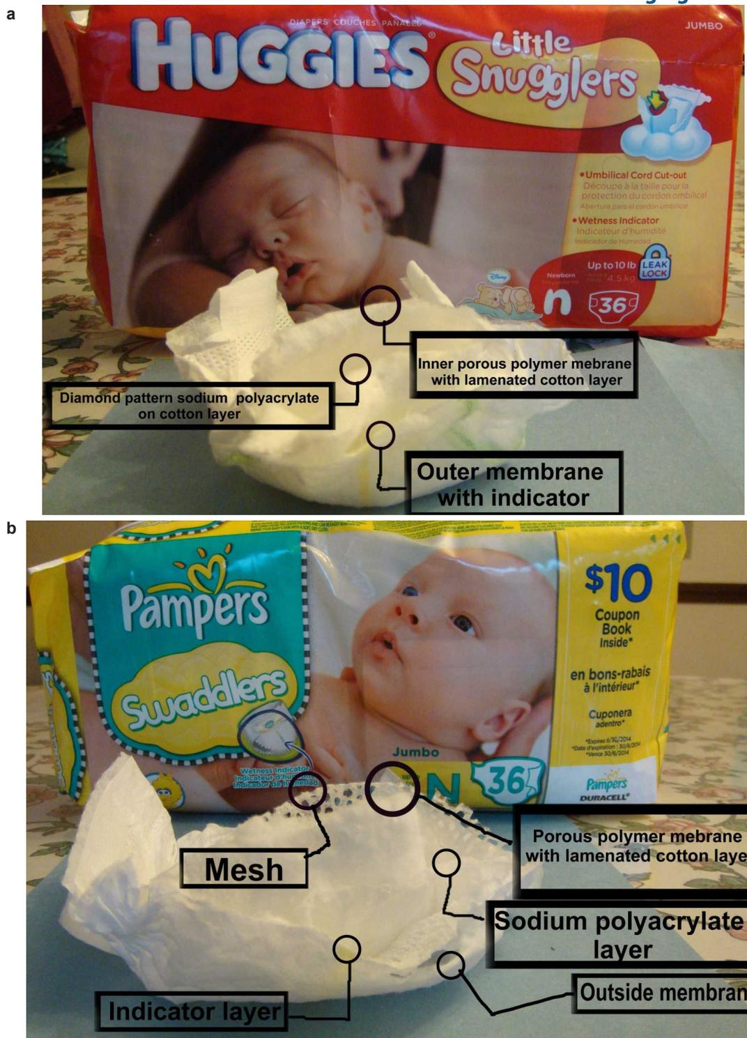
Figure 1. Cross-section of Diaper. (a) Huggies' Cross-section. (b) Pampers' Cross-section.
