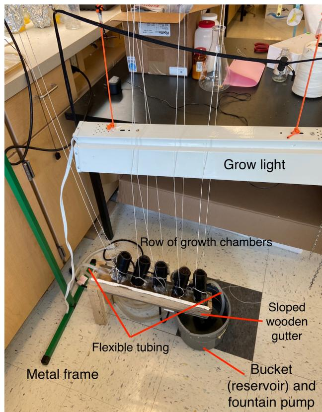
**Figure 6: Experimental setup.** This labeled image shows the entire setup of the experiment. It shows how each component was hung from the metal frame, as well as the setup of the gutter system to ensure that a consistent water flow was delivered to one end of each choice chamber.
