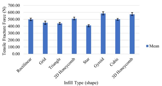
**Figure 2:** Means for each infill type. Gyroid infill had the highest mean tensile fracture force while the star shape had the lowest. Error bars indicate the range of tensile forces for each infill pattern. An ANOVA analysis showed a *p*-value of 3.3405E-18.
