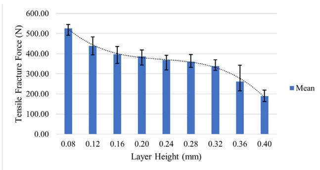
**Figure 3:** Means for each layer height. The 0.08 mm layer height had the highest mean tensile fracture force, while 0.40 mm had the lowest mean. As the layer height increased, the mean tensile fracture force decreased. Error bars indicate the maximum and minimum tensile forces for each layer height. The dotted line shows a cubic regression curve with an  $R$ -value of 0.9972. An ANOVA analysis showed a  $p$ -value of 2.3660E-17.
