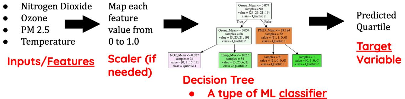
**Figure 1: Flow chart illustrating the steps for machine learning classification.** Shows the features passed in as inputs to the classifier, which then predicts the ED visits quartile (target).
