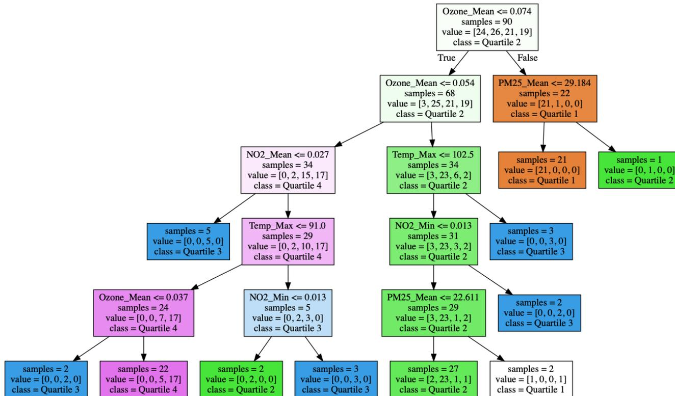
**Figure 2: Mean O<sub>3</sub> yielded the greatest separation of classes in the decision tree model.** A graphical tree (.dot file) is shown from the decision tree classifier. The separation of classes for various features are represented. The nodes higher in the tree provided greater separation.
