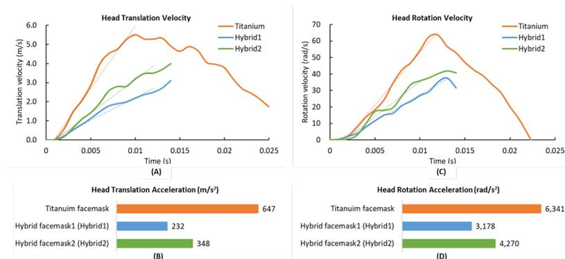
**Figure 8. Head velocity curves and head acceleration.** (A)(C) Dashed lines show linear regressions of the head velocity over 0.01 s. Hybrid1 and Hybrid2 show a slower increase of the head velocity than Titanium facemask for both the translational and rotational head velocities. (B)(D) Head acceleration comparison.
