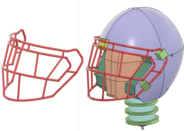
**Figure 9. Head-neck and football helmet model.** Fusion 360™ model: Facemask is 3-dimensionally modeled.
