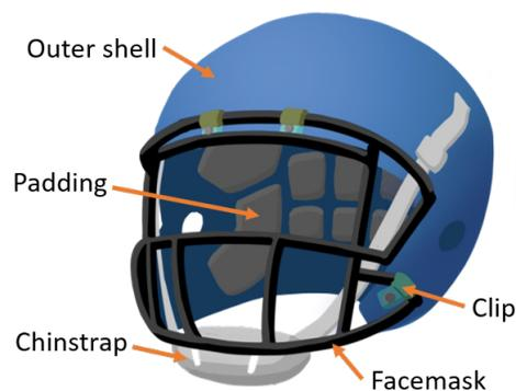
**Figure 1: American football helmet.** Facemask is mounted on the front and made of steel or titanium. Outer shell, chin strap, and clips are plastics. Padding is soft foam or rubber.
