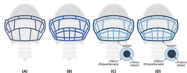
**Figure 4. Facemask designs.** (A) Titanium facemask and Polycarbonate facemask 1 (PC1). (B) Polycarbonate facemask 2 (PC2). (C) Hybrid facemask 1 (Hybrid1). (D) Hybrid facemask 2 (Hybrid2).
