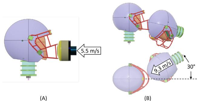
**Figure 3: Simulation condition.** (A) Ram impact test with a 5.5 m/s ram speed to the front of the helmet. (B) Helmet-to-helmet collision with a 9.3 m/s strike helmet speed with 30° attack angle.
