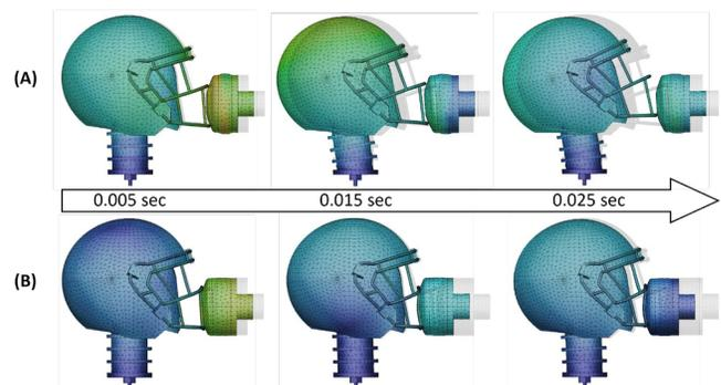
**Figure 5. Ram impact test simulation result.** (A) Titanium facemask. (B) PC1. PC1 shows less head translation by the ram impact with larger deformation. Countour shows velocity.
