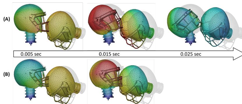
**Figure 7. Helmet-to-helmet collision simulation result.** (A) Titanium facemask. (B) Hybrid2. Hybrid2 facemask result is limited to 0.015 seconds due to a computational time constraint in the software. Angled attack generates both translation and rotation of the head. Hybrid2 facemask reduces the translation and rotation of the head. Contour shows velocity.
