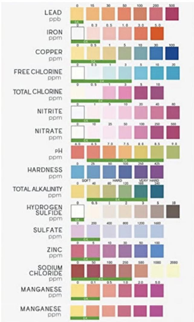
**Figure 6. Color chart for parameter testing.** The resolution guide is provided by the Varyfy water test kit website (16). Results were taken by comparing color change on the strips with the colors shown in this figure.
