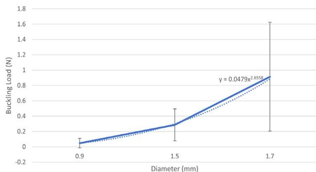
Figure 1. Buckling load (N) increased with diameter of pasta (mm). Buckling load was measured using homemade system for spaghetti-like pasta of three diameters. Data points are fitted with an exponential function and a dotted line of best fit has been shown. Error bars on the y-axis show the standard deviation of the buckling load for each point.
