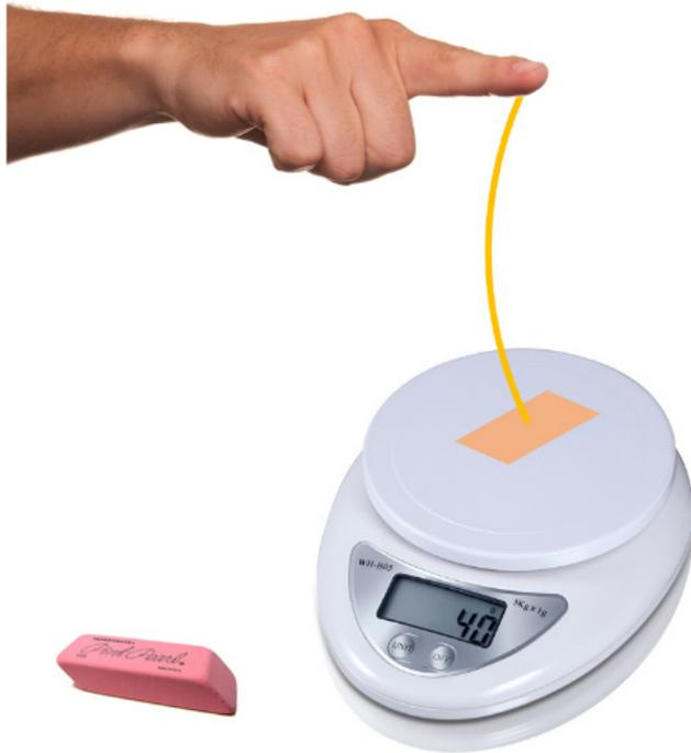
**Figure 3. Experimental setup of buckling experiment for reference.** The setup included masking tape, scissors, a weighing scale, ruler, eraser (to be used as a cushion between the finger and pasta if needed), and spaghetti of different diameters.
