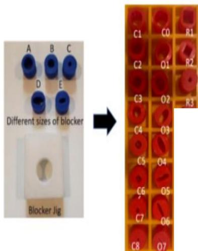
**Figure 5: Bronchial blockage models tested.** Blockages were labeled Cx, Ox, Rx, with x being a number with bronchi diameter decreasing as x increases. The C, O, and R labeled the shapes circle, oval, and rectangle respectively.
