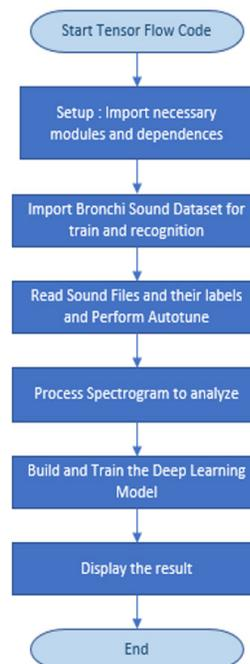
**Figure 6: Flow chart representing the implementation of Deep Learning.** Tracks the steps from start of TensorFlow code to the display of the result after analyzing the sound files.
