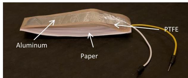
**Figure 8. Aluminum, paper, and PTFE based TENG.** This is a contact-separation mode TENG made to evaluate the effects of using different negatively charged materials in a TENG. In this generator, PTFE is the negatively charged material, paper is the positively charged material, and aluminum is the conductive surface.
