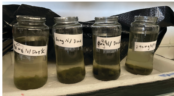
Figure 3: Jars with no algal pretreatment in a dark environment. Four jars containing river water with nitrate added at the following concentrations, from left to right: 0, 133, 400, and 1200 ppm, were kept in complete darkness to inhibit algal growth. The same algal biomass shown in Figure 2 (primarily blue-green algae, likely cyanobacteria such as Anabaena or Microcystis spp., though not taxonomically confirmed) was added to each jar. This photo was taken on Day 9, immediately before the algae were filtered out and fish were introduced. The jars were kept under identical conditions except for light exposure; no light source was provided in this setup.
