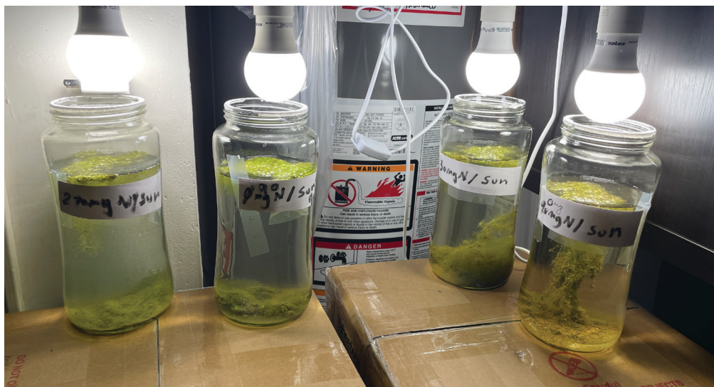
Figure 2: Jars with added algal pretreatment in a light-rich environment. Four jars were kept under daylight bulbs (40-watt each) to promote algal growth. The jars contained river water with nitrate added at the following concentrations, from left to right: 0, 133, 400, and 1200 ppm. Each jar included algal biomass consisting mainly of blue-green algae (likely cyanobacteria such as Anabaena or Microcystis spp.), though no formal identification was performed. This photo was taken on Day 9, immediately before the algae were filtered out and fish were introduced.
