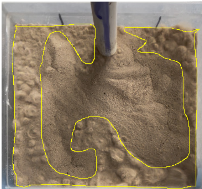
Figure 5. Representative fluidized bed at 1% water saturation. 12.5 g of water was mixed with 1250 g of dry sand, and 1250 g of dry sand was layered on top of the mixture. 90 PSI of air was injected into the bed (18.5 cm by 21.0 cm). The large, encircled area in yellow shows the fluidized area captured by this photo (181.52 cm 2 ). Other photos at this water saturation level captured fluidized areas of 192.09 cm 2 and 190.05 cm 2 and exhibited similar fluidized behavior (n=3).
