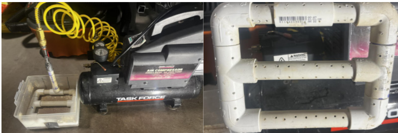
Figure 8. Fluidized bed setup and bottom of PVC network. A polyvinyl chloride (PVC) network was placed in a transparent container, which received air from an air compressor. 84 holes with a 2.38 mm diameter were drilled on the bottom roughly 10 mm apart. The holes on the three main pipes on separate sides were 90 degrees apart from one another, and holes were drilled in a similar fashion on the curves of the PVC network.
