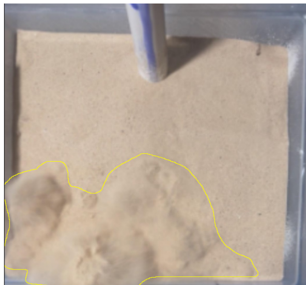
Figure 4. Representative fluidized bed at 0.5% water saturation. 6.25 g of water was mixed with 1250 g of dry sand, and 1250 g of dry sand was layered on top of the mixture. 90 PSI of air was injected into the bed (18.5 cm by 21.0 cm). The encircled yellow area represents the fluidized area captured by this photo (140.66 cm 2 ). Other photos at this water saturation level captured fluidized areas of 130.93 cm 2 and 136.93 cm 2 and exhibited similar fluidized behavior (n=3).
