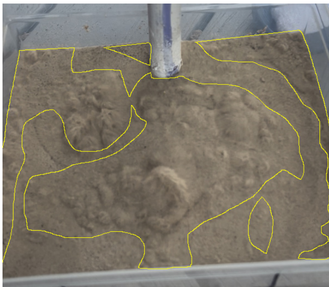
Figure 3. Representative fluidized bed at 0% water saturation. No water was present in the fluidized bed composed of 2500g of sand. 90 PSI of air was injected into the bed (18.5 cm by 21.0 cm). The encircled yellow area represents the fluidized area captured by this photo (321.81 cm 2 ). Other photos at this water saturation level captured fluidized areas of 325.14 cm 2 and 345.87 cm 2 and exhibited similar fluidized behavior (n=3).
