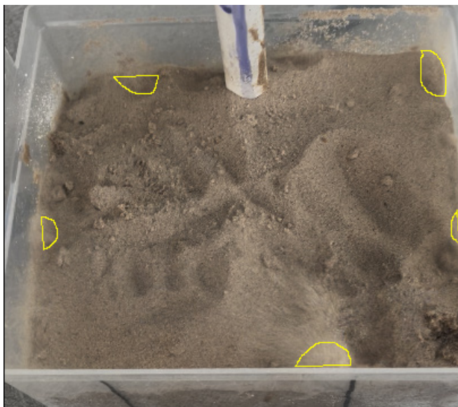
Figure 7. Representative fluidized bed at 60% water saturation. 750 g of water was mixed with 1250 g of dry sand, and 1250 g of dry sand was layered on top of the mixture. 90 PSI of air was injected into the bed (18.5 cm by 21.0 cm). The small yellow circles in the photo represent the fluidized area that exhibited slugging (10.19 cm 2 ). Other photos at this water saturation level captured fluidized areas of 10.02 cm 2 and 11.14 cm 2 and exhibited similar fluidized behavior (n=3).
