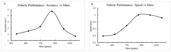
Figure 3: Vehicle Mass Effect on Accuracy and Speed. (A) The average (A) accuracy (m<sup>-1</sup>) and (B) speed (m/s) of (specify) was measured for 6 different weights of a gravity vehicle (507, 627, 747, 867, 987, and 1107 g).
