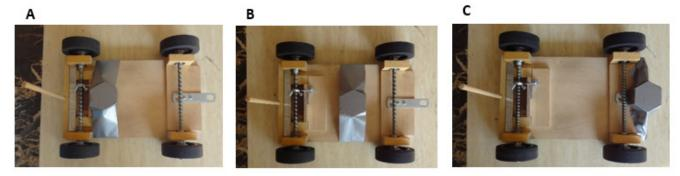
Figure 1: Gravity Vehicle with Different Mass Loading. (A) The front load was located behind the front axle due to the dowel in front of the axle. (B) The load was located at the middle point of the vehicle length, and the load behind the rear axle. All three load configurations were located on the center line and secured with duct tape to prevent movement during the run.
