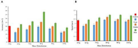
**Figure 2:** Effect of CG Location on Accuracy and Speed. The average (A) accuracy (m<sup>-1</sup>) and (B) speed (m/s) of (specify) was measured for 6 different weights of a gravity vehicle (507, 627, 747, 867, 987, and 1107 g) as the load was moved from the front (blue), middle (orange), and rear (green) of the vehicle. Measurements were compared to an unloaded vehicle as a control (red) (n = 3). Error bars represent two standard deviations.
