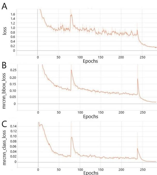
**Figure 2. Tensorboard Loss Statistics following Model Training.** Loss is defined as the difference between the results of the ground-truth “user” annotation training data and the model’s prediction attempt. Pictured here: segmentation loss (A), binding-box loss (B), and class loss (C). Segmentation and binding-box identifies coral features while class loss predicts which class those features belong to healthy or diseased coral.
